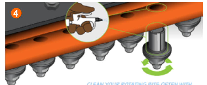
CLEAN YOUR ROTATING BITS OFTEN WITH COMPRESSED AIR TO REMOVE GRIT & DUST. THEY MUST SPIN FREELY FOR BEST PERFORMANCE & LONG LIFE.
